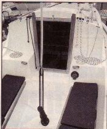
Cockpit features drip-dry cushions and fixed mainsheet take-off point on floor.
